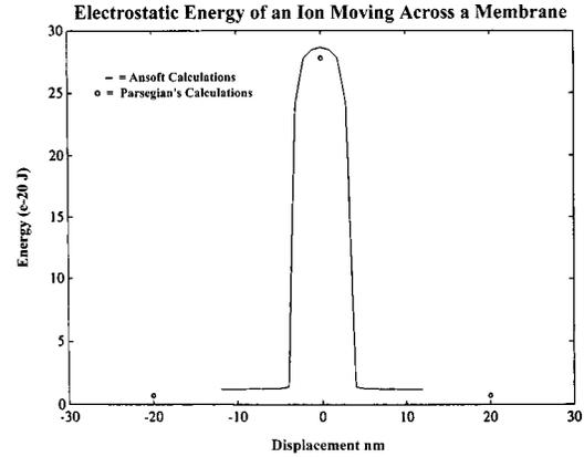
Fig. 3. Estimate of the lipid bilayer barrier [77]. Energy barrier for charge insertion based on the electrostatic energy change as a singly charged ion is moved from water into and across a bilayer membrane of thickness 6 nm.
