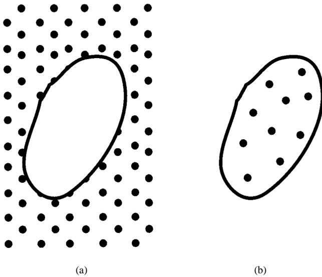
Fig. 2. Illustration of molecular uptake by electroporation. The irregular central object is a cell. (a) High extracellular concentration of a fluorescent molecule (solid ellipsoidal dots). (b) Nonequilibrium concentration of fluorescent molecules inside cell after a single electroporating pulse, membrane recovery, and removal of the extracellular supply solution [75], [76].
