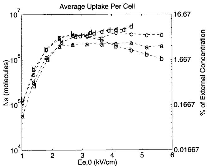
Fig. 10. Calcein uptake versus single pulse magnitude for yeast cells [82]. In spite of a very heterogeneous response, above  $\sim 2.5\text{ kV/cm}$  the measured uptake is  $\bar{n} = (1.5 \pm 1) \times 10^6$  molecules cell $^{-1}$ , about 2.5% of the equilibrium value.
