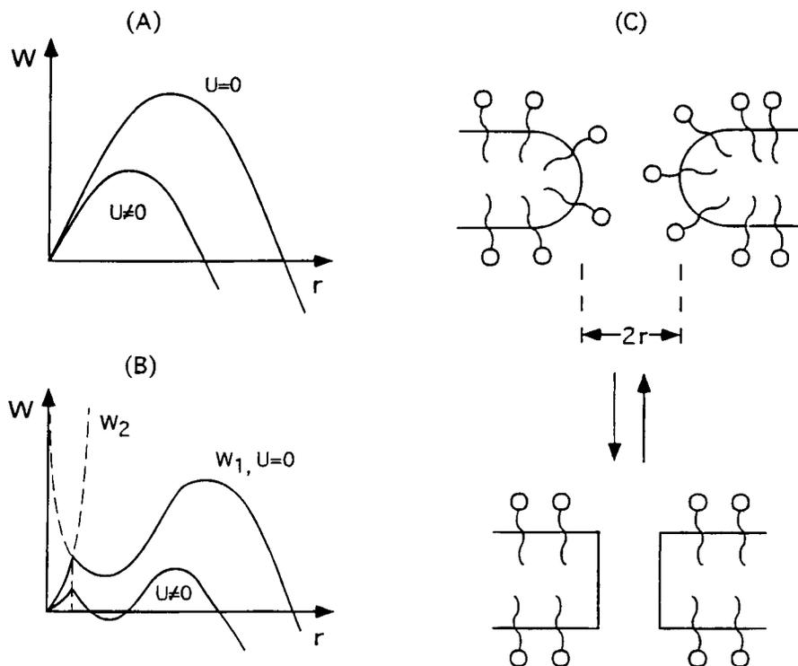
Fig. 5. Pore creation free energy change [7]. A transition from hydrophobic pores (lower right) to hydrophilic pores (upper right) is hypothesized, with a strong, nonlinear dependence on the local transmembrane voltage.
