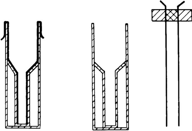
Fig. 1. Typical *in vitro* electroporation apparatus. Cross-sectional drawing of a cuvette with parallel plane metal electrodes for pulsing a cell suspension.
